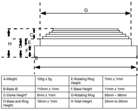
"G" - The actual shape of the target dome is to be engineered to provide the best aerodynamic design and flight stability.
