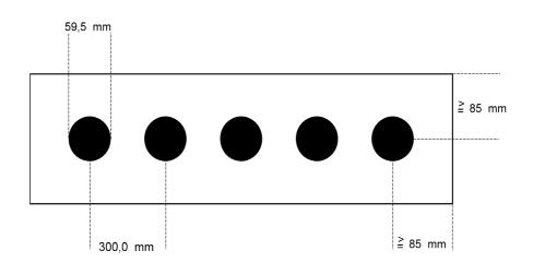
The Diameter of the black is 59.5 mm with a tolerance of +0.2 mm / -0.0 mm
